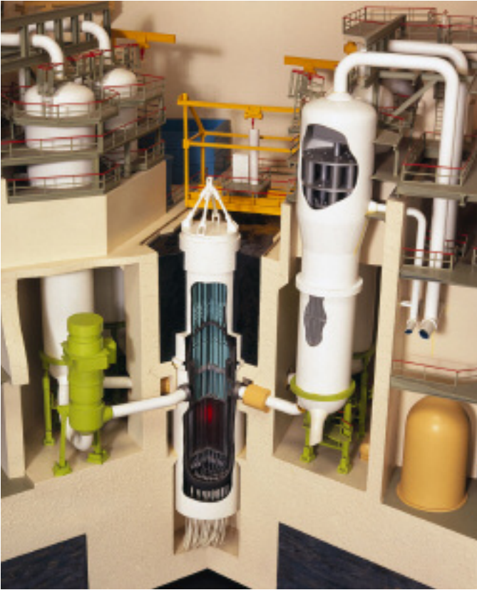
Figure 3. An engineering model of the Pressurised Water Reactor at Sizewell B. Photo: Science Museum/SSPL.
