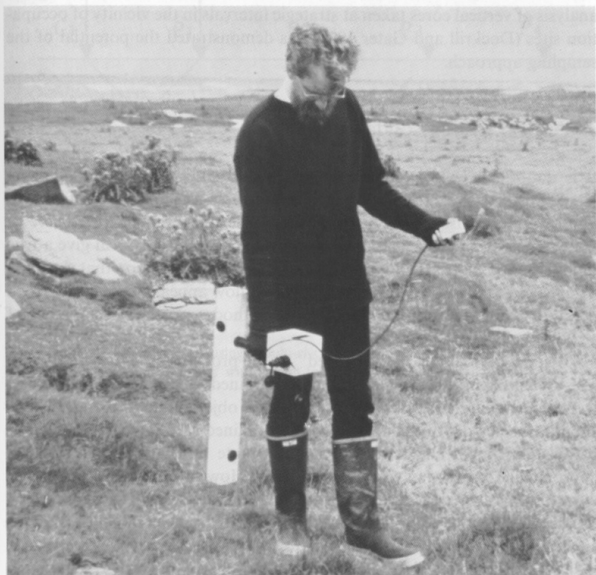
Figure 4. Rapid magnetic surveying with the FM18 fluxgate gradiometer.
