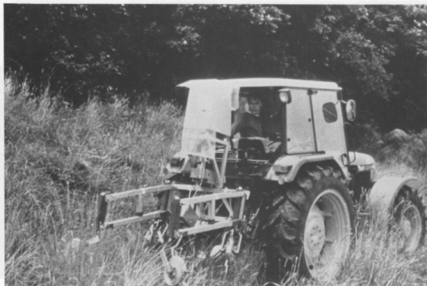
Figure 3. Continuous earth resistance measurements with the RATEAU system and a mobile "square" array.
